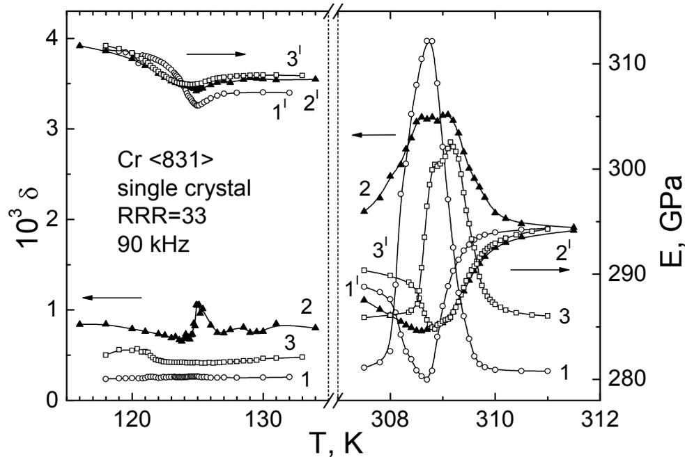
Fig. 5. Effect of plastic deformation on the dependences  $\delta(T)$  (curves 1 to 3) and  $E(T)$  (curves 1' to 3') in the vicinity of the Néel point and the spin-flip transition:  $\circ$  – undeformed specimen,  $\blacktriangle$  – after a plastic deformation,  $\varepsilon_{pl} = 1\%$ , at room temperature,  $\square$  – after plastic deformation,  $\varepsilon_{pl} = 1\%$ , and subsequent ageing at room temperature for 1 year.
