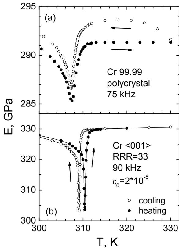
Fig. 2. Acoustic anomalies on the temperature dependences  $E(T)$  near the Néel point in the Cr polycrystal (a) and  $\langle 001 \rangle$  single crystal (b) [2] at thermocycling with a heating-cooling rate 0.1 K/min.
