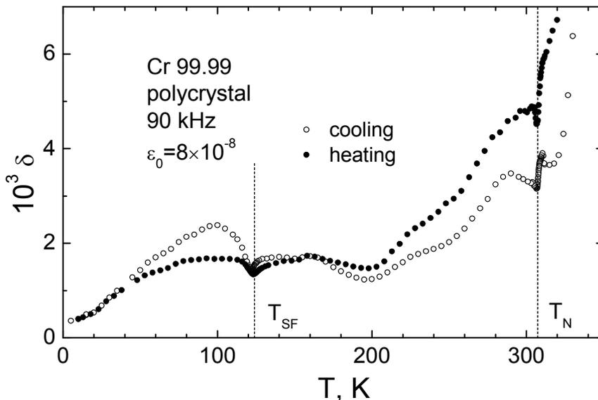
Fig. 3. Hysteresis in the temperature dependence of the decrement  $\delta(T)$  in a polycrystalline sample measured at a frequency of 90 kHz:  $\circ$  – cooling,  $\bullet$  – heating.
