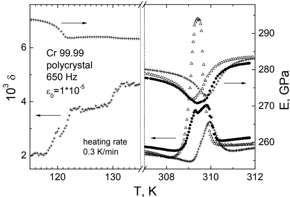
Fig. 4. Effect of heat treatments on the behavior of the decrement and the Young's modulus near the Néel point and variation of the low-frequency acoustic properties in the vicinity of the spin-flip transition: ● – after quenching from 1273 K, + – after quenching from 1523 K, Δ – after quenching from 1273 K and subsequent annealing at 733 K for 2 hours.
